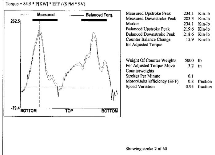
Figure 8 - Dynamometer After Gas Separator Installation
