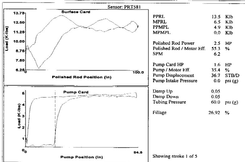
Initial Dynamometer Test
