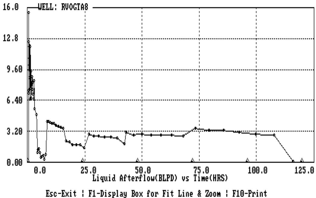
Figure 6 –Liquid Afterflow vs. Time
