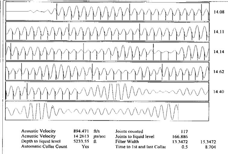
Figure 7 – Acoustic Test After Installation of Gas Separator
