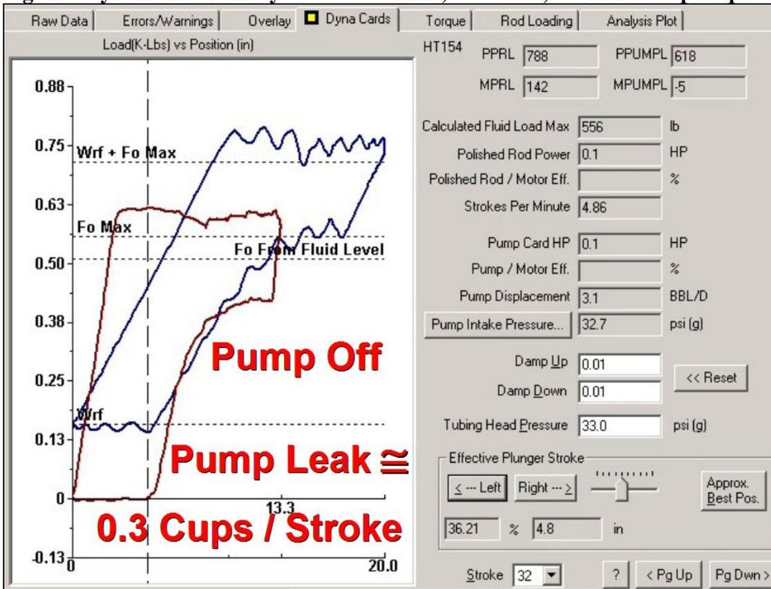
**Figure 12 – Inches of Surface Stroke Lost to Stretch of Rods Picking Up Fluid Load**
