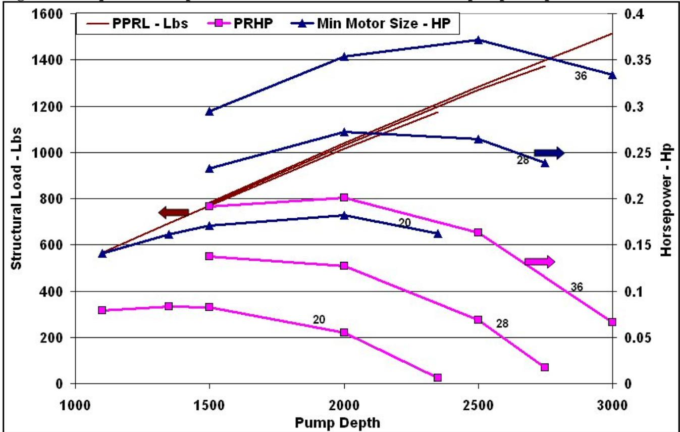
Figure 5 – Pump Displacement for Standard Sized LVPS for Pump Depths Up to 3000 Feet
