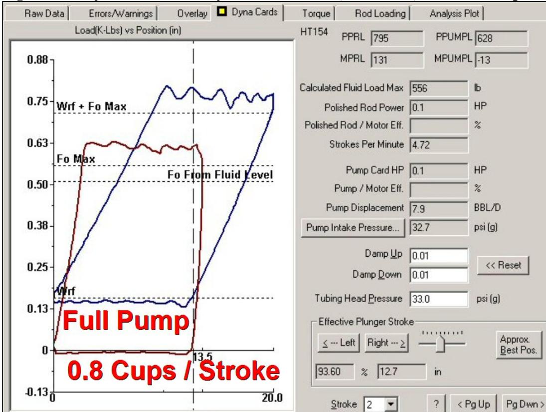
**Fig. 11 - Dynamometer Analysis ~ 0.055 PRHP, 4.86 SPM, 3.1 BPD Pump Displacement**
