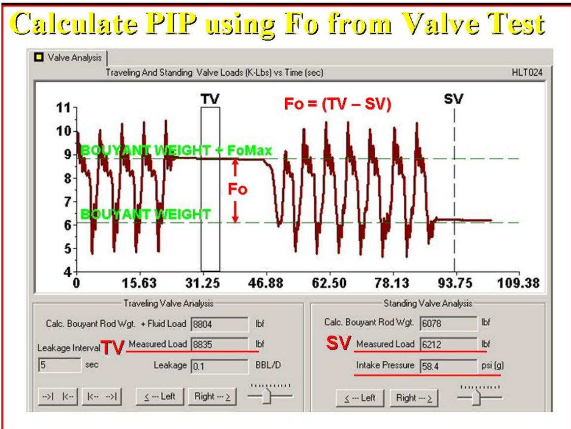
Figure7 – Sample valve Test showing measured values used in calculation of PIP
