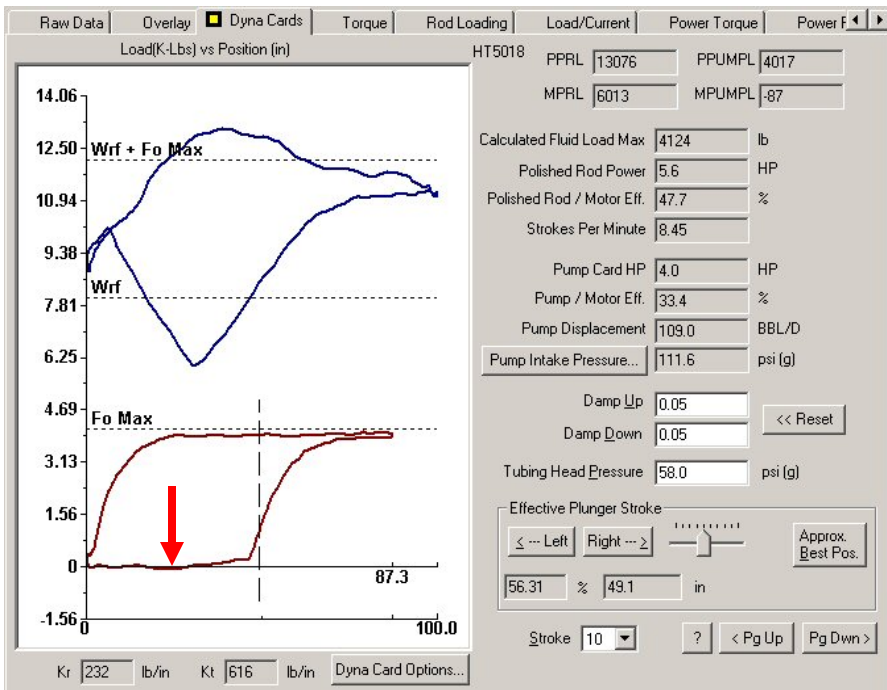
Figure 4 Surface and Pump Plunger Dynamometer Cards and Analysis
