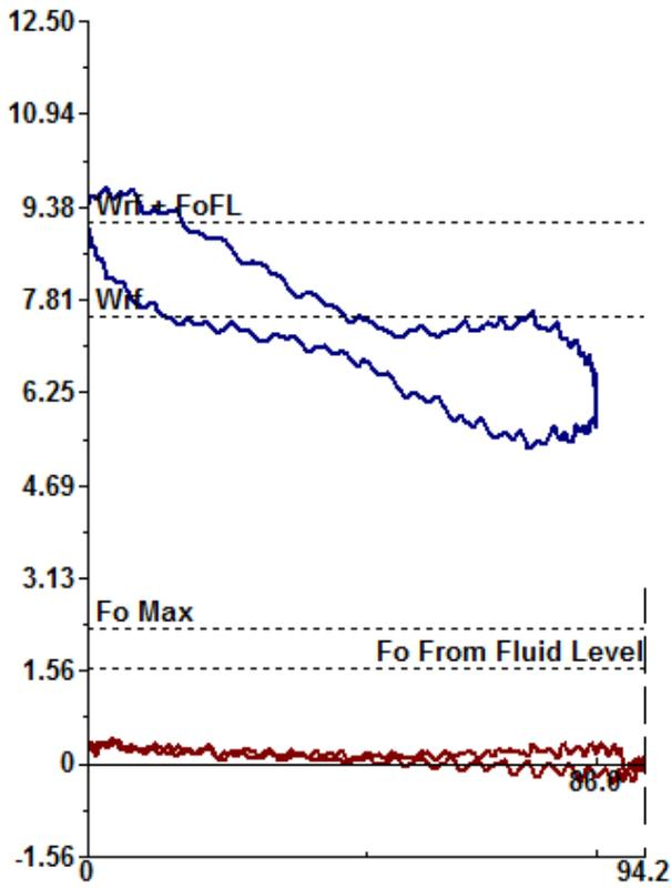
Figure 6 – Tubing Liquids Unloaded by Gas
