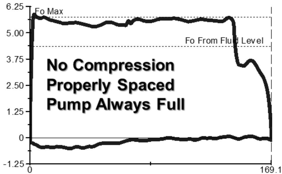
Figure 4 – Tag the Pump to Open TV at Bottom of Stroke
