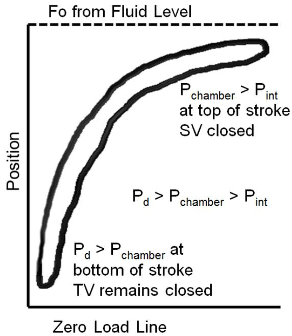
Figure 2 – Pressure Relationship for Gas Filled Pump Chamber from Intake to Discharge Volume
