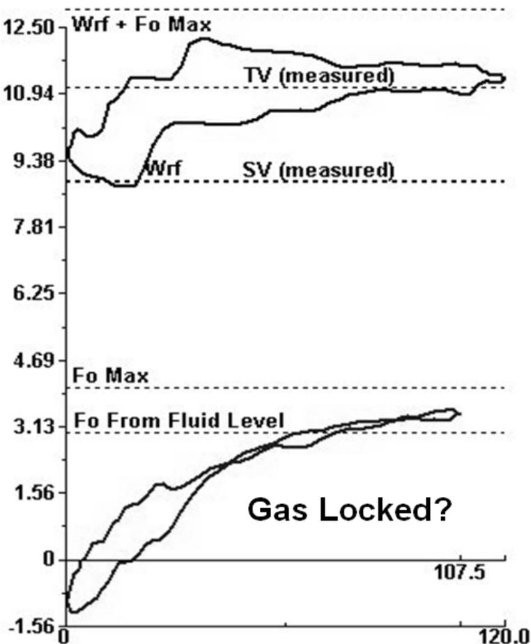
Figure 5 – TV Open Pump Card Showing No Pump Action
