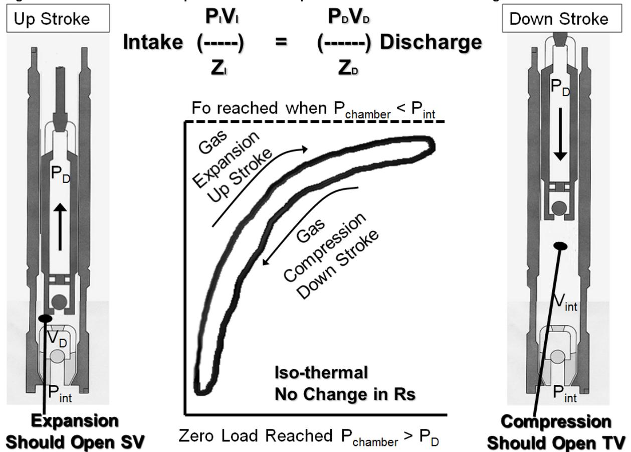
Figure 3 – Variable Slippage Pump Filled with Liquid as Free Gas Discharged at top of Up Stroke
