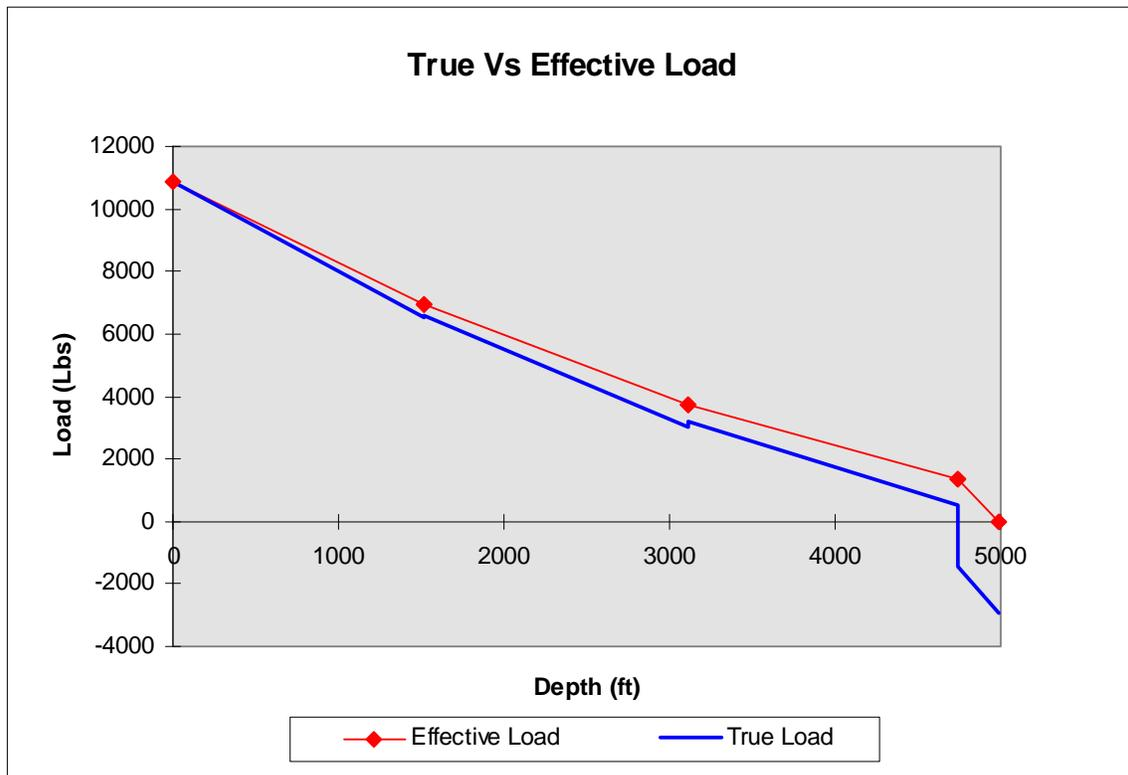
Figure 3 – True Vs. Effective Load from DHLC (205i03.csv) File (Red – 0.75 Dia. Rod)
