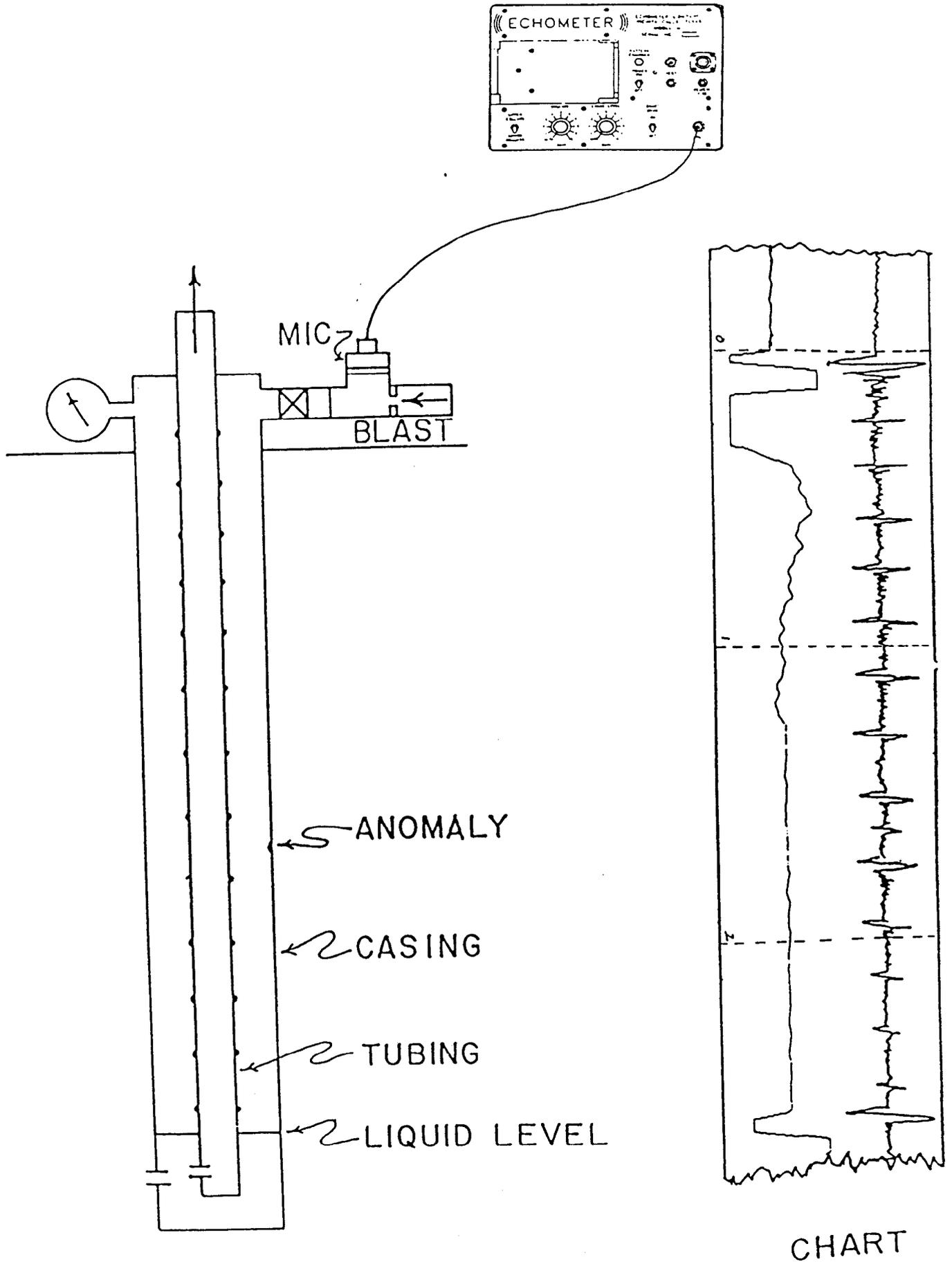
Figure 1 Acoustic Liquid Level System
