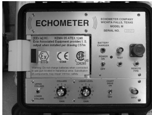
Figure 3 - Model M Acoustic Fluid Level Instrument that has been modified, as shown by the engraving, to include safety circuits to limit electrical energy output in the event of a component malfunction and using the manual gas guns listed above with the model E installed in a safe area.
