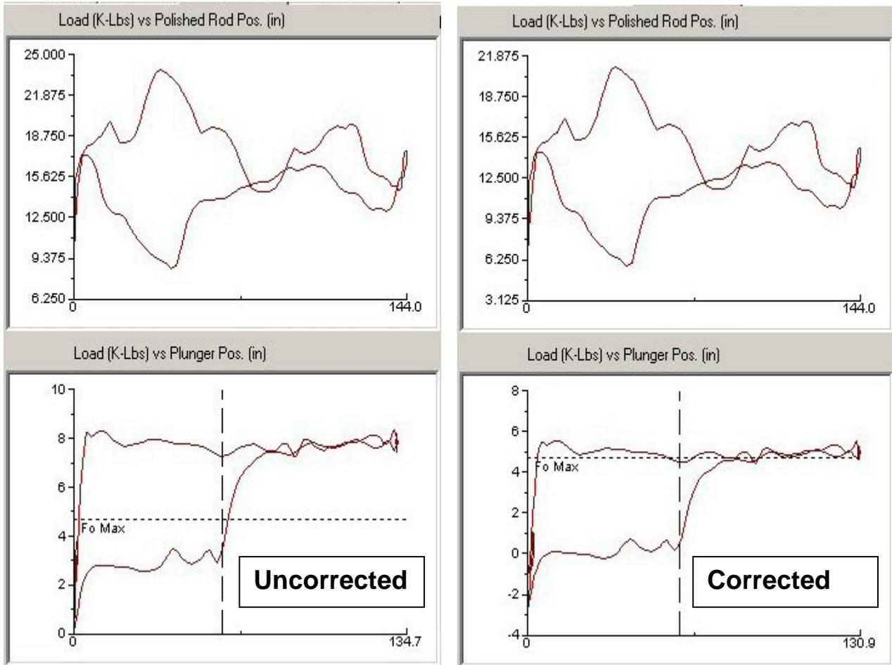
Fig. 9 – Comparison of Polished Rod and Pump Dynamometer Cards for PRT and Load Cells
