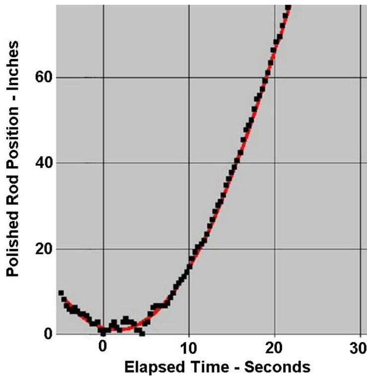
Fig. 4 – Polished Rod and Plunger Position Versus Elapsed Time for Anchored Tubing.
