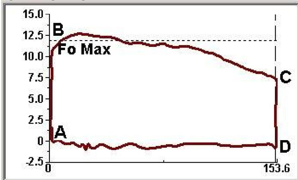
Fig. 7 – Pump Card with Unaccounted Friction from Paraffin
