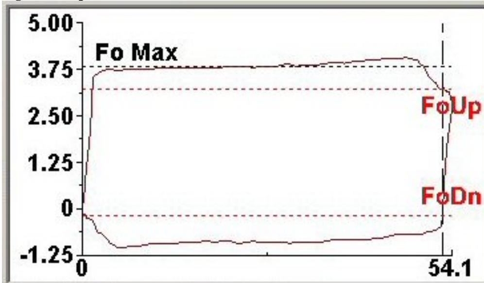
**Fig. 8 – Surface PRT Dynamometer Adjusted for Load Offset due to Tagging on the Down Stroke**
