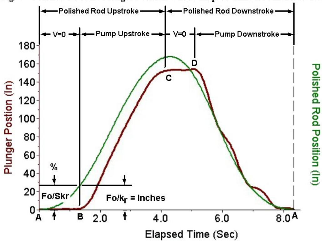
Fig. 5 – Polished Rod and Plunger Velocity Versus Elapsed Time for Anchored Tubing.
