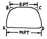
Leaking traveling valve, TV, or excessive plunger slippage causes delay in picking up fluid load from A to B and premature unloading from C to D, (the traveling valve, TV, is effective only during a portion of the upstroke).
