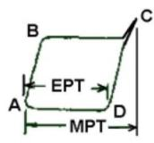
Practically any combination of the malfunctions shown above may exist in any well. The effects of these malfunctions may be superimposed on one another and the combined effect may be masked. For instance, the presence of gas interference and a tubing anchor that is has become unseated may exhibit a card whose individual effects may not readily be evident. The tubing stretch constant, K<sub>t</sub>, superimposed on the card may afford an insight into the problem.
