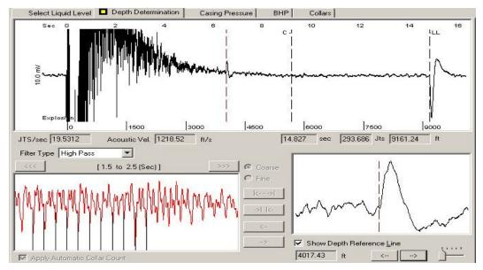
An anomaly in the annulus above the liquid level was detected at a depth of 4017 feet, as indicated by a strong reflected rarefraction (up kick) acoustic pulse recorded at 6.507 seconds. The anomaly was displayed at the same depth in both acoustic traces collected while testing the well. The depth to the anomaly corresponds very well to the increase in the casing volume at the depth of 4015.92 at the crossover from the 2 3/8 inch Hydril to the 1.90 inch Hydril collar-less tubing.
