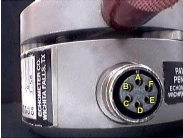
If the measured readings are not within 25% of these stated values, then you should send the Horseshoe Transducer Load Cell in to Echometer for repair.
