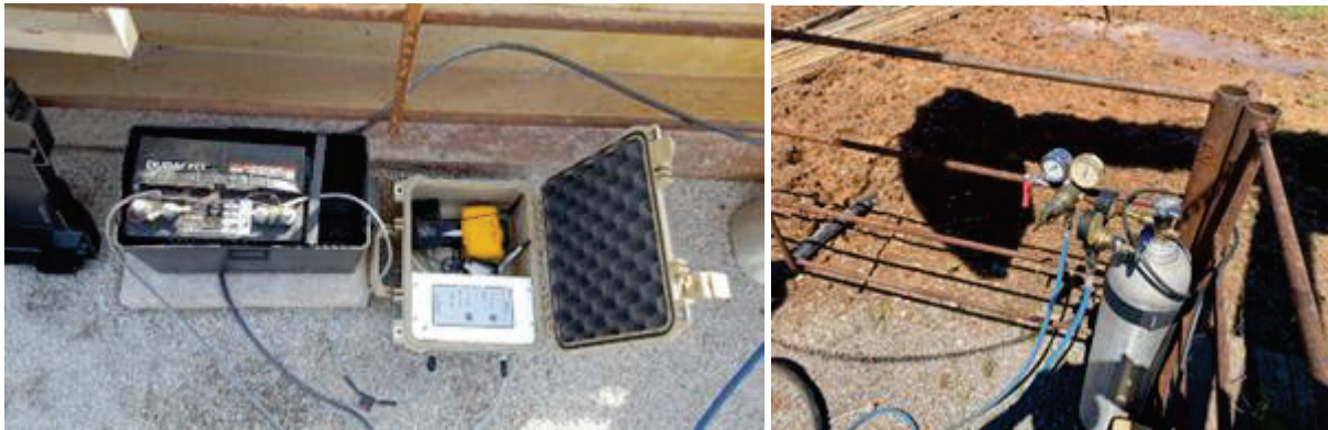
Figure 4: RAM box connected to external battery and Nitrogen supply for long term operation.
