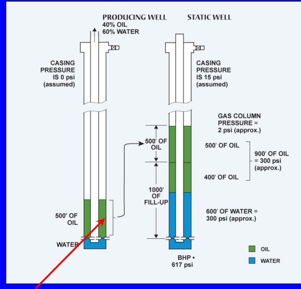
Need to compute % of oil and water in annulus at end of fill-up period.
