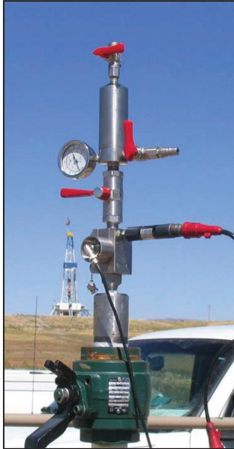
For best results, before attaching the gun to the wellhead, replace any needle valves with ½ inch ball valves in order to minimize energy loss through connection as shown below:
