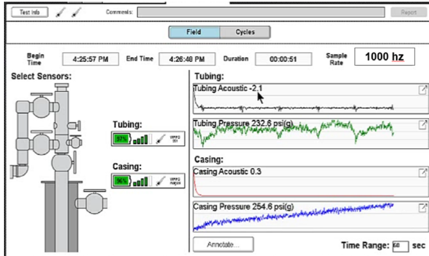
Figure 7 – Wireless equipment streaming data in plunger tracking software
