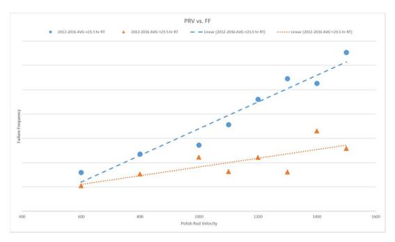
Figure 6: Polished Rod Velocity vs. Failure Frequency
