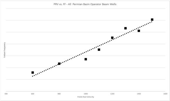
Figure 5: Plot of PRV v FF for all Operator Permian Basin beam wells
