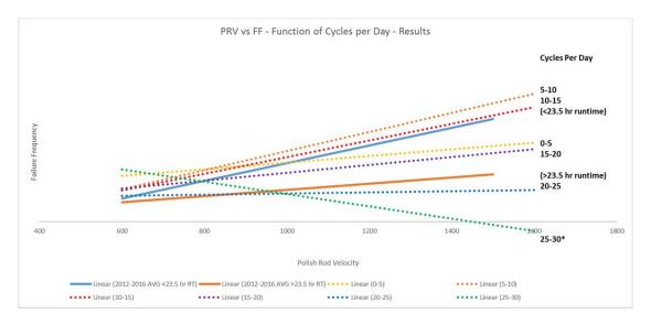
Figure 11: Polish Rod Velocity vs Failure Frequency as a function of Number of Cycles Per Day
