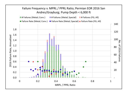
Figure 1: Failure Frequency, Shallow San Andres/Grayburg (dots indicate failure rates on left Y-axis, bars indicate number of failures on right Y-axis)
