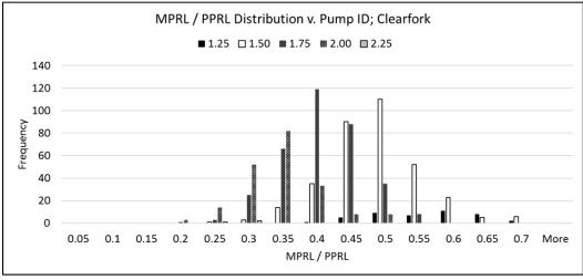
Figure 4: MPRL/PPRL Distribution for Clearfork Wells by Pump Size
