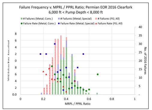
Figure 2: Failure Frequency, Moderate Depth Clearfork (dots indicate failure rates on left Yaxis, bars indicate number of failures on right Y-axis)
