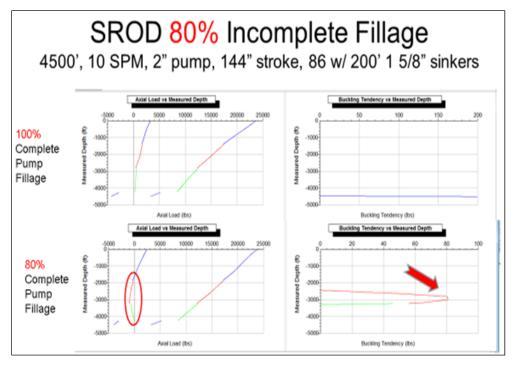
Figure 9: Complete Pump Fillage vs. 80% Pump Fillage
