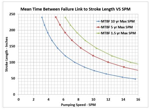
Figure 8: Relationship Between Stroke Length, Pumping Speed, and MTBF
