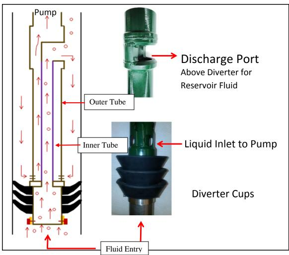
Figure 6 shows a schematic diagram of the Diverter Separator and pictures of some of its principal components.
