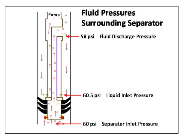
Figure 8 – Estimated pressure distribution for a field installation.
