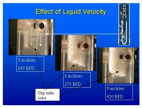
Figure 3 Gas entrainment into the separator dip tube at increasing rates
