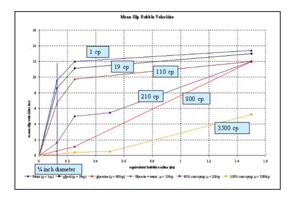
Figure 2 Air bubble slip velocities in liquids of different viscosity
