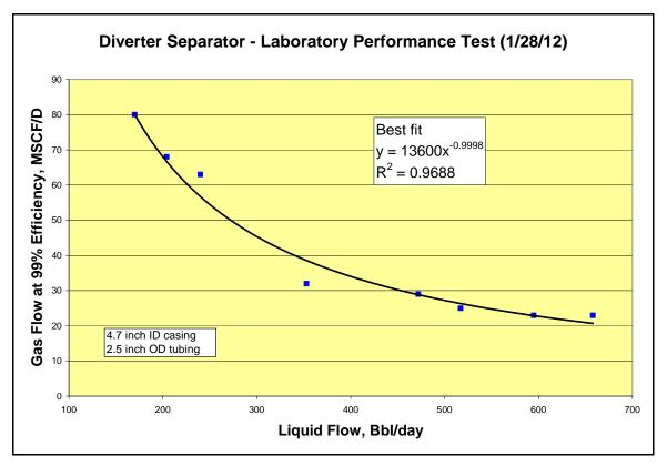
Figure 7 – Typical Laboratory Test Results for 5 inch pipe.
