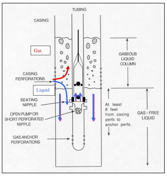
Figure 4 Natural gas-liquid separator
