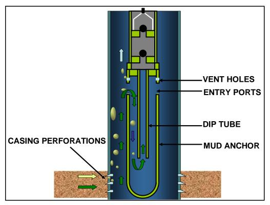
Figure 1 Downhole gas-liquid separator
