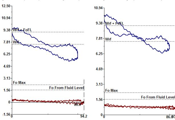
Figure 5 – TV Open Pump Card Showing No Pump Action
