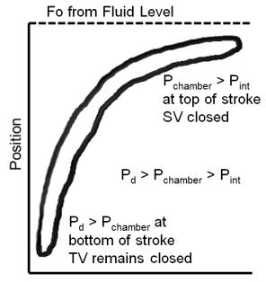
Figure 1 – Diagnostic Gas Locked Pump Card Shape
