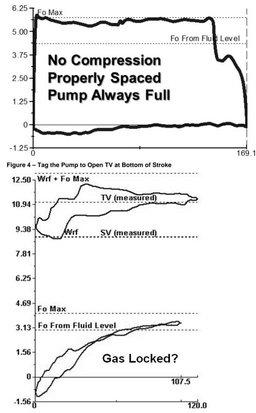
Figure 3 – Variable Slippage Pump Filled with Liquid as Free Gas Discharged at top of Up Stroke
