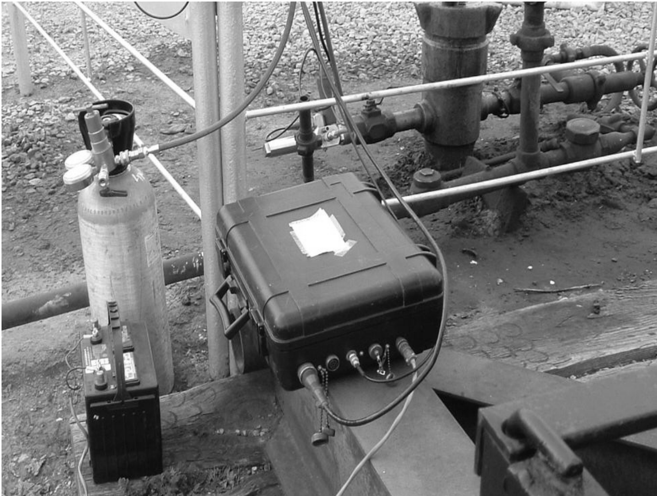
Figure 1 – Acoustic liquid level set-up for programmed automatic operation
