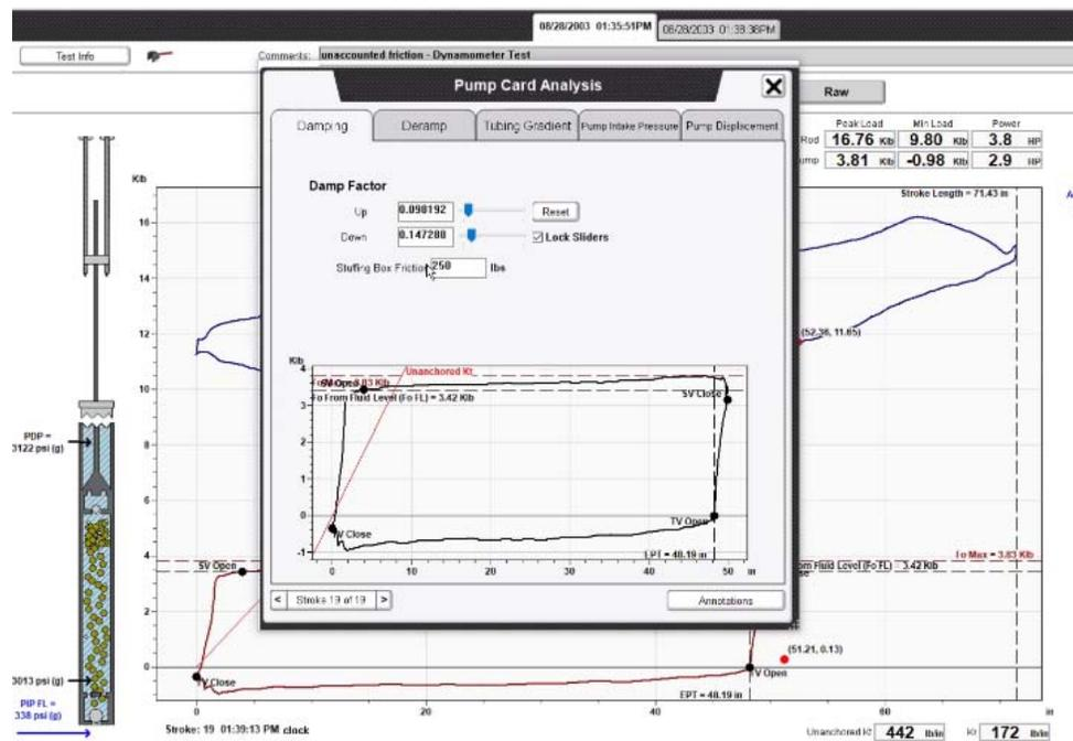
If the pressure on top of the plunger, and the intake pressure below the plunger aren't changing during the upstroke, then the load line is going to be flat if you have the right fluid dampening removed. If the pressure is changing throughout the stroke, the load line won't be flat.
