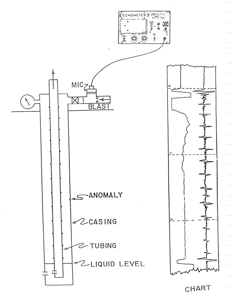
Figure 1 Acoustic Liquid Level System
