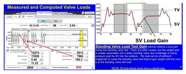
We don't calculate it in TWM or TAM. Slide 38 shows a leaky standing valve. The change in load vs. time represents how fast the rods unstretch. If rods stretch due to the load changing we COULD calculate it, we just don't.
