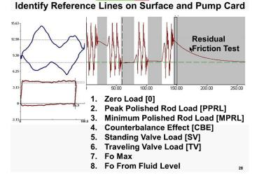
During the time when the fluid load is dropping off from the TV load to the SV load, as shown in the final TV test on slide 28, at some point along that time when performing the CBE test, when you release the brake the loads won't move up or down. That is the point that describes the effect of the weights and the crank because the loads will be in balance.
