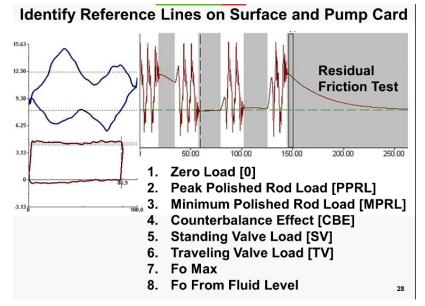
The unit was probably not stopped as well on the second test. If you jerk the brake and stop it too fast then some of the traveling valve load is picked up. This is actually fluid load on the downstroke on the rodstring because the traveling valve moved down, and picked up some load and then it leaks off. You can see it drops slightly on the second test. If we had let it sit longer it would have dropped off to the same level.
