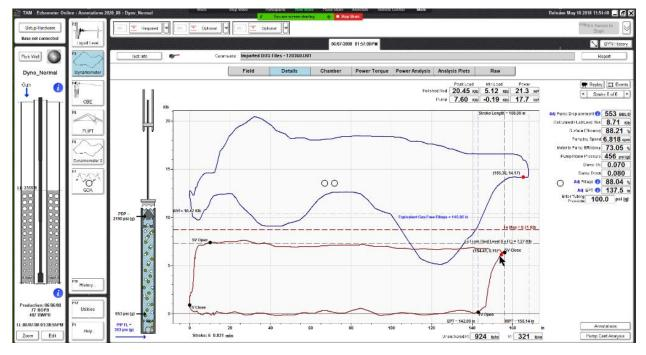
The shape on the downstroke (arrow) is gas compression. The difference between the EPT and Gas Free Pump Fillage line is the free gas in the pump when the traveling valve opens. And the length from the Gas Free Pump Fillage line to the MPT line represents how much free gas entered the pump chamber. So you see a compression curve if you have incomplete pump fillage on the right hand side of the pump card.
