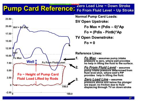
The surface stroke is 168 inches, and the pump stroke is 156 inches. The pump stroke length is less due to the stretch from picking up the fluid load.
