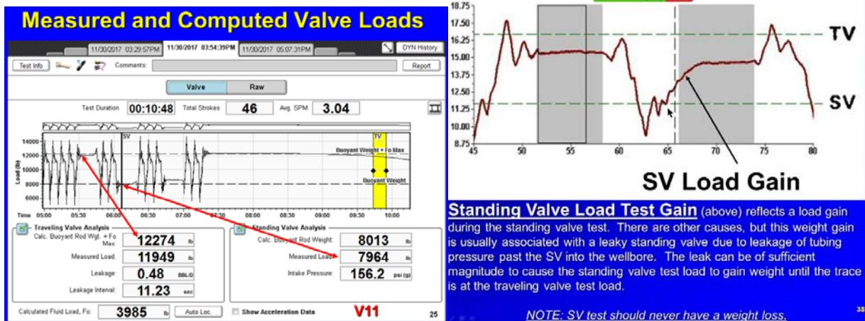
We don't calculate it in TWM or TAM. Slide 38 shows a leaky standing valve. The change in load vs. time represents how fast the rods unstretch. If rods stretch due to the load changing we COULD calculate it, we just don't.
