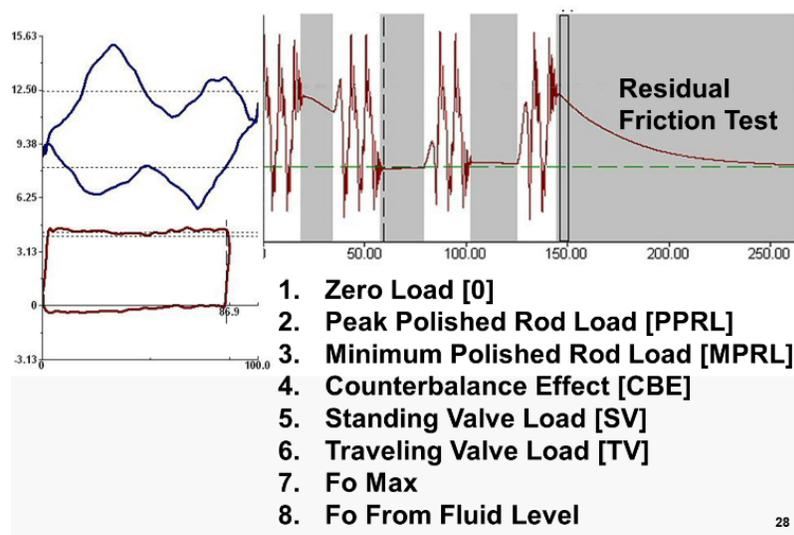
The unit was probably not stopped as well on the second test. If you jerk the brake and stop it too fast then some of the traveling valve load is picked up. This is actually fluid load on the downstroke on the rodstring because the traveling valve moved down, and picked up some load and then it leaks off. You can see it drops slightly on the second test. If we had let it sit longer it would have dropped off to the same level.
