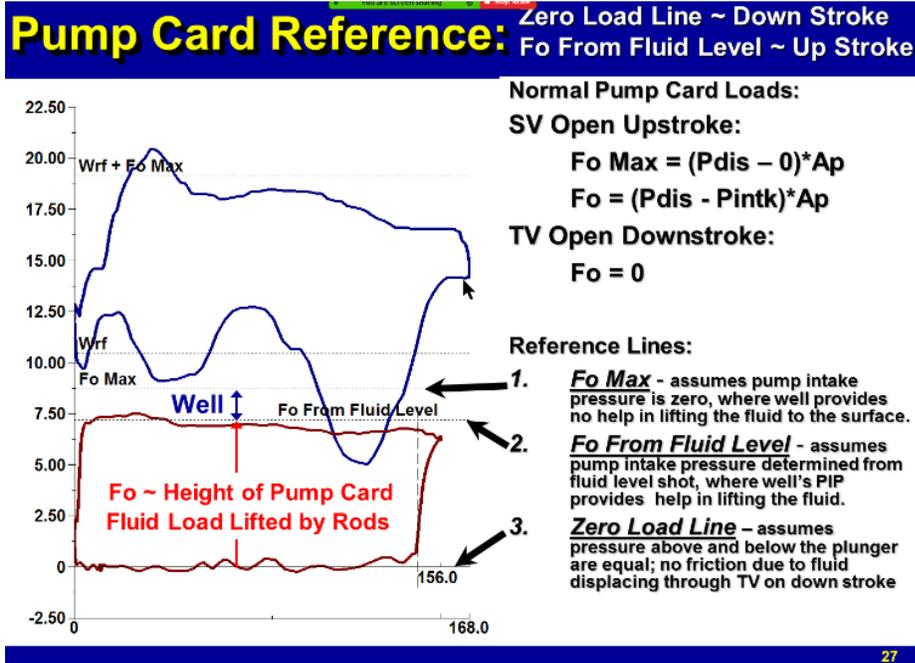
The surface stroke is 168 inches, and the pump stroke is 156 inches. The pump stroke length is less due to the stretch from picking up the fluid load.
