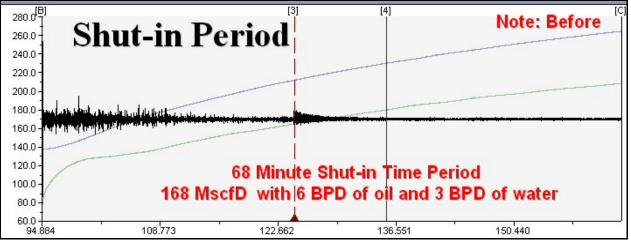
Figure 17 – Shut-in Time Period Adjusted to Minimum Time
