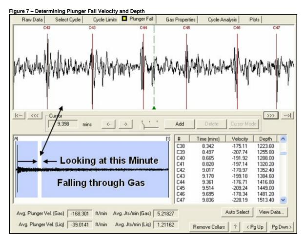
Figure 8 – Plunger Fall Velocity and Depth
