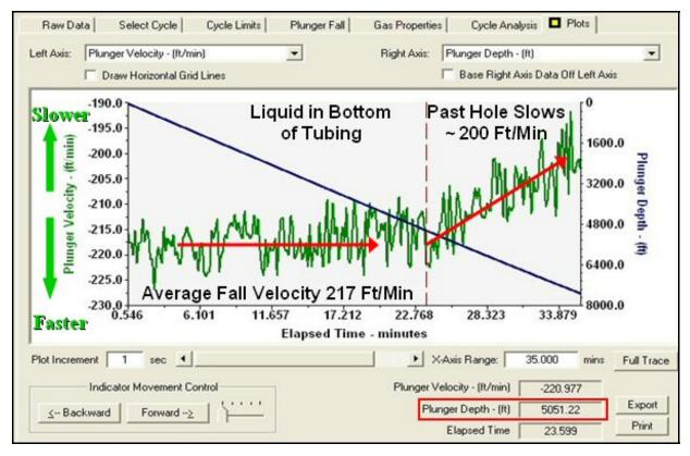
Figure 14 – Tubing Pressure Change Increases when Plunger Passes Hole in Tubing
