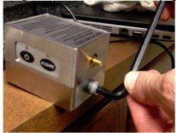
3. Place a ½" cap on the threads to completely seal the W5KG opening. The ½" Test Cap will not be a sufficient seal because the rubber bulb could be blown off with the pressure pulse when the gun is fired.
