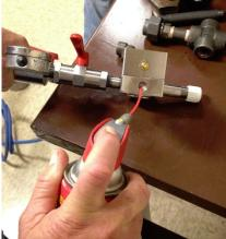
6. Attach a ¼" street elbow pipefitting or a hose (see picture below) in the ¼" Bleed Plug hole. Wrap the threads with Teflon tape before attaching to prevent galling, and for easier removal from the Housing.
