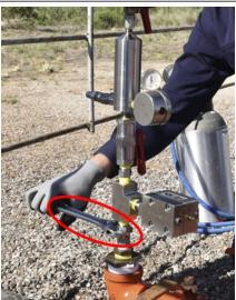
Prepare the gas gun to perform a Zero Offset measurement of the Pressure Transducer in the gun.
