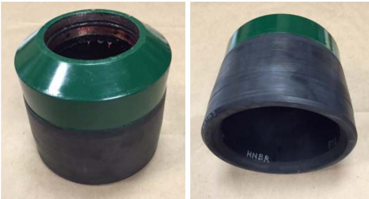
Figure 7 – Special Design Flow Isolator cups are used to control flow in the casing annulus.
