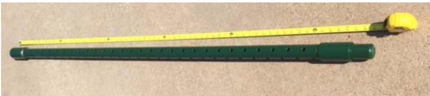
Figure 11 Perforated sub for installation at bottom of Tail Pipe.
