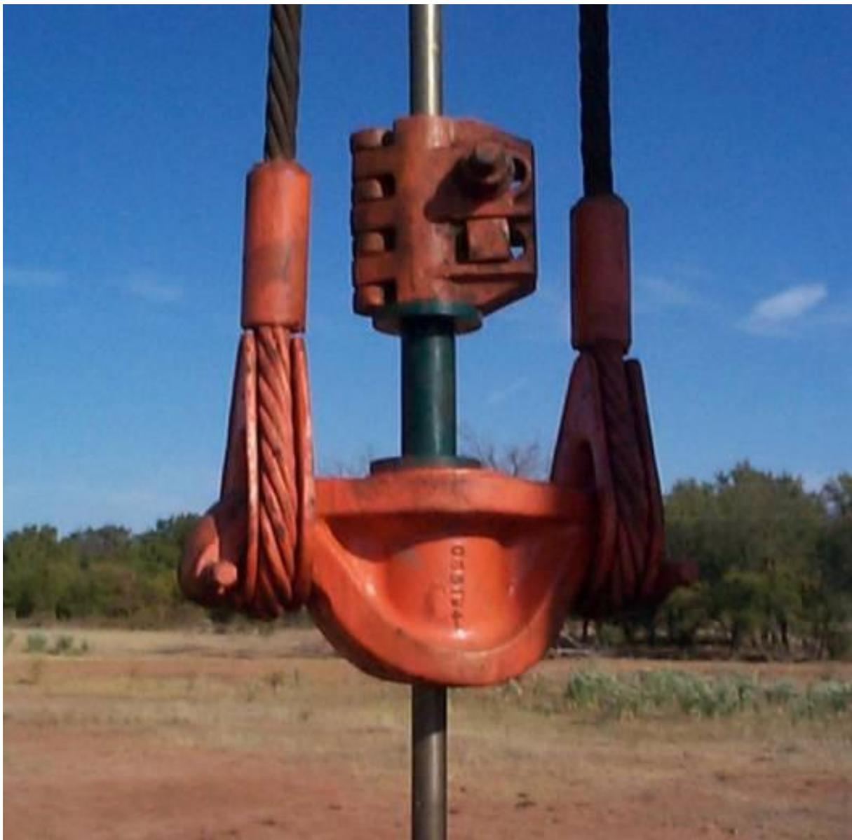
To install the 50k horseshoe transducer and hydraulic jack and spacer, the pumping unit is stopped at the bottom of the downstroke.
