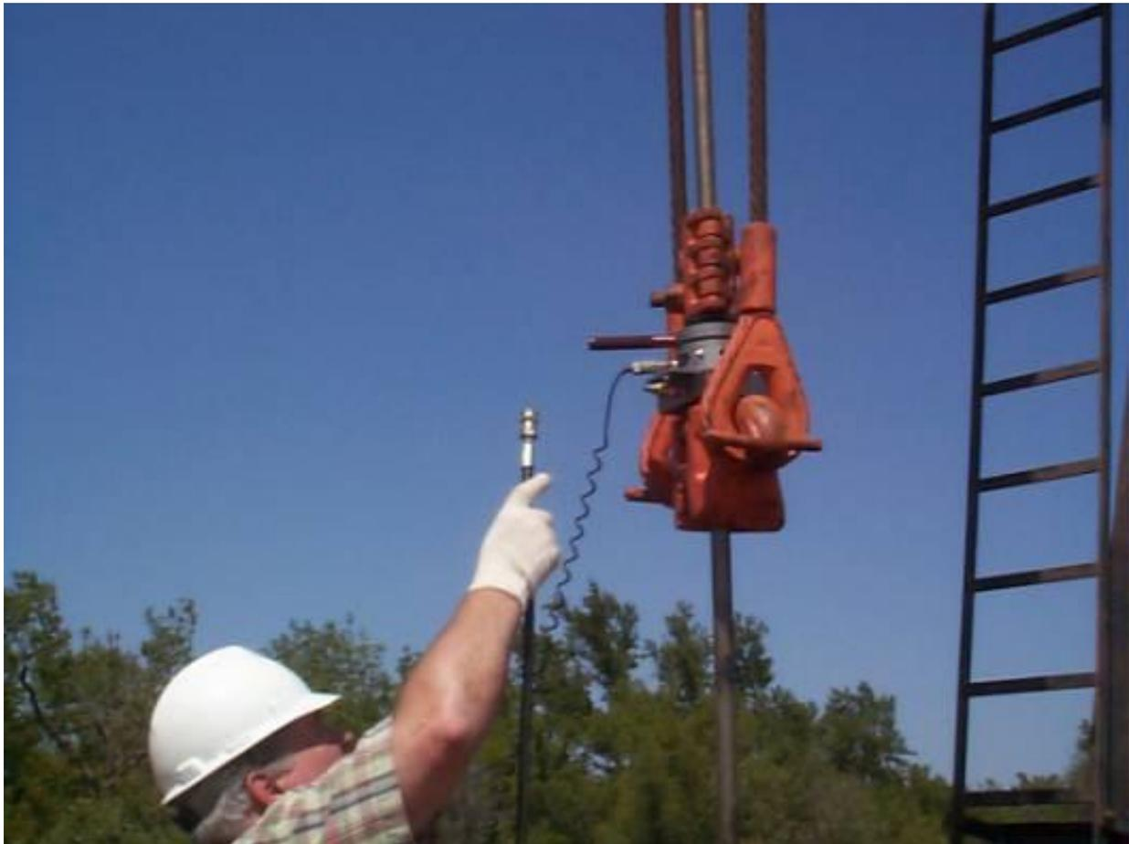
A cable is attached from the Well Analyzer to the horseshoe transducer to record accurate polished rod load and also acceleration data.
