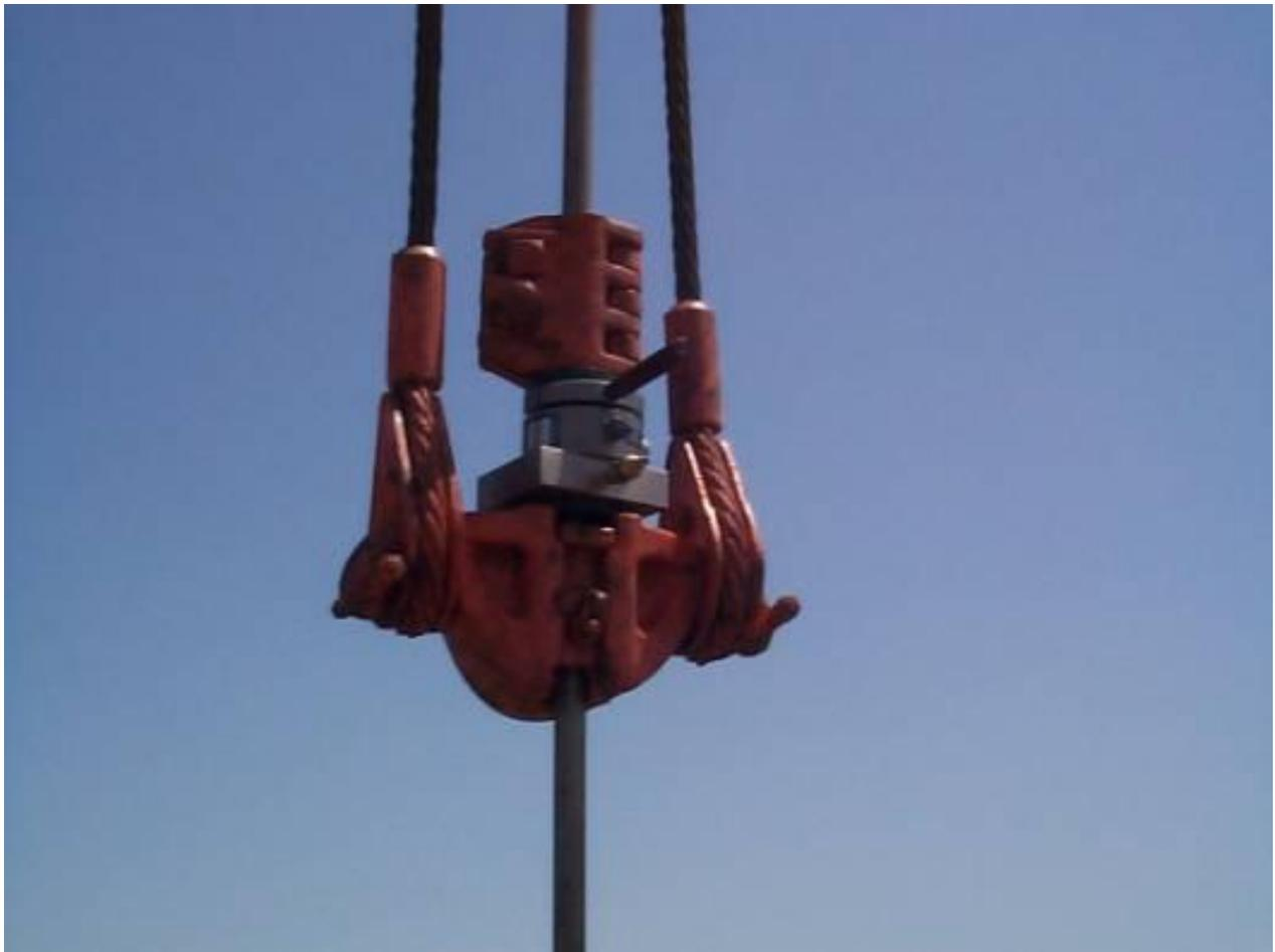
The hydraulic pump is actuated to raise the horseshoe transducer and place the polished rod load onto the horseshoe transducer.
