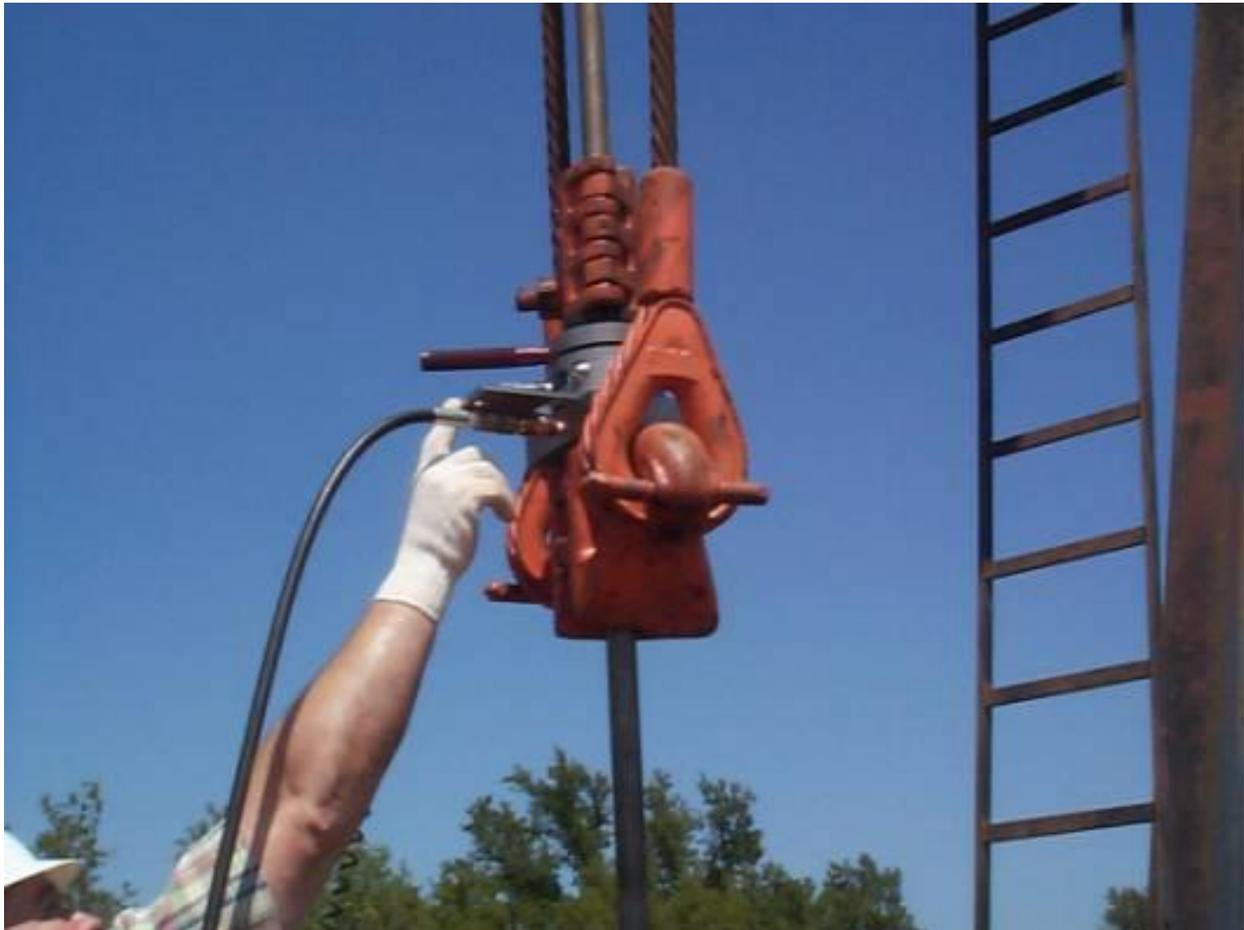
After the spacer is inserted, the hydraulic liquid is bled back into the pump, and the polished rod load is lowered onto the horseshoe transducer, spacer plate, and the hydraulic jack. The entire polished rod load is on the horseshoe transducer.
