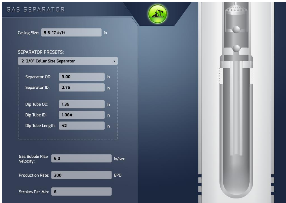
Figure 6 – Simulator Input Screen for Definition of Gas Separator Dimensions and Pumping System and Fluid Properties.
