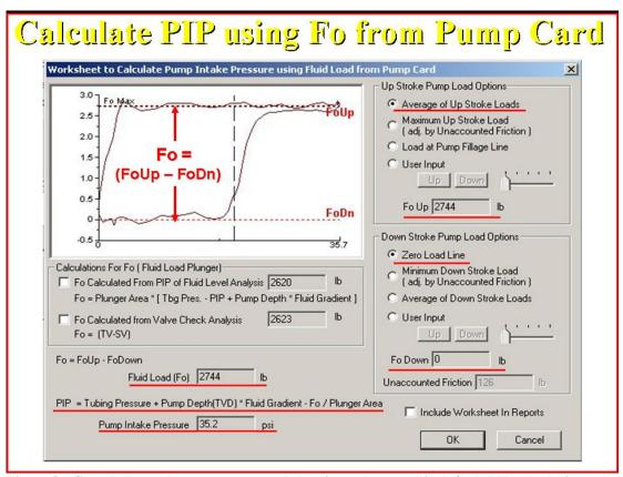
Figure 8 - Sample Pump Dynamometer card showing values used in default PIP calculation
