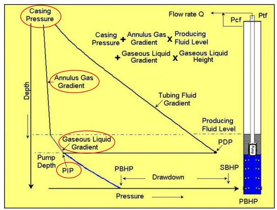
Figure 1 – Definition of Pump Intake Pressure from Acoustic Fluid Level Survey
