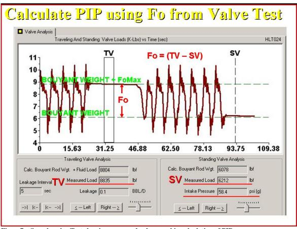
Figure7 - Sample valve Test showing measured values used in calculation of PIP
