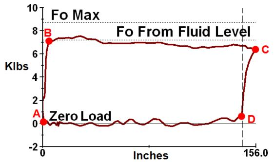
Figure 2 – Resulting Pump Displacement Calculated using QRod - TTU Slippage Test 0.005 Clearance 76 Rod String 7.045 SPM File Tools Help
