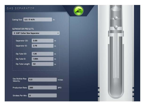
Figure 6 – Simulator Input Screen for Definition of Gas Separator Dimensions and Pumping System and Fluid Properties.
