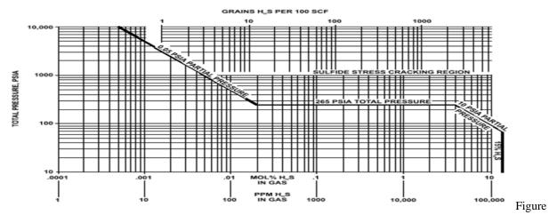
1. NACE MR0175 prior edition chart to determine potential for material to sulfide stress crack. (Ref. 2) Table I. NACE MR0175/ISO 15156 Table on Exceptions
