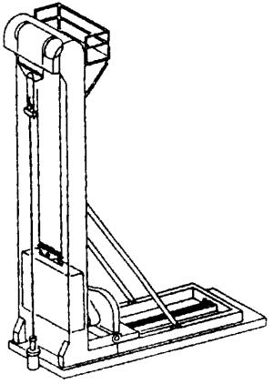
Figure 2 – RotaFlex Chain Drive
