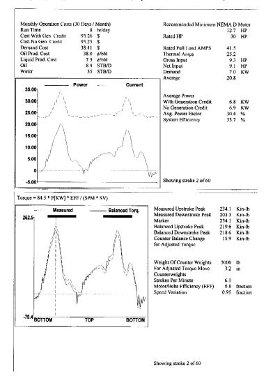
Figure 8 - Dynamometer After Gas Separator Installation
